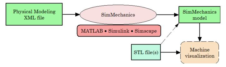
From an XML multibody description file to a Simscape Multibody Model
