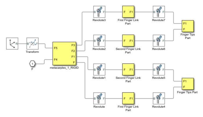
Multibody Simulink Subsystem with Body Simulink Subsystems
