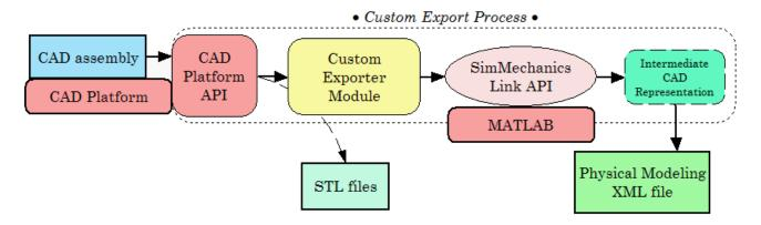
Custom Export: From a CAD Assembly to an XML Multibody Description File
